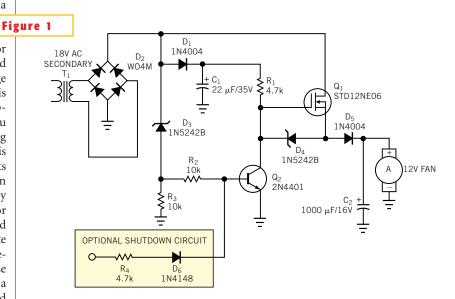
Using a MOSFET circuit, you can efficiently convert the too-high voltage of a leftover transformer to a lower dc level.
